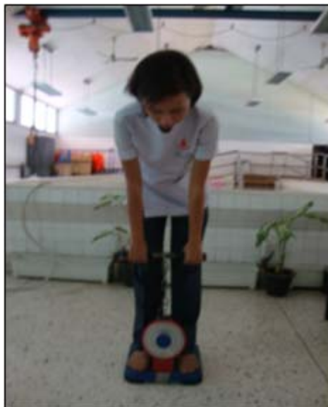
Figure 2. Back-leg dynamometer for measuring back muscle strength.
