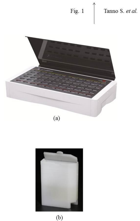
Figure 1 Examination unit of the DOX system (a). The unit interfaces with a personal computer. DOX coliform cassette (b).
