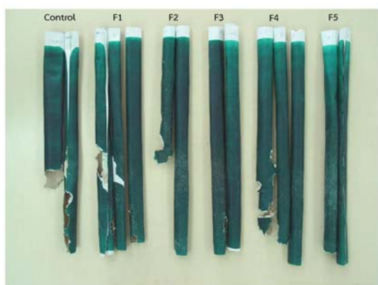
Figure 5 The example of cardboard sprayed with ink mixed with various repellents after 24-hour exposed to the rats in the circular open field.
