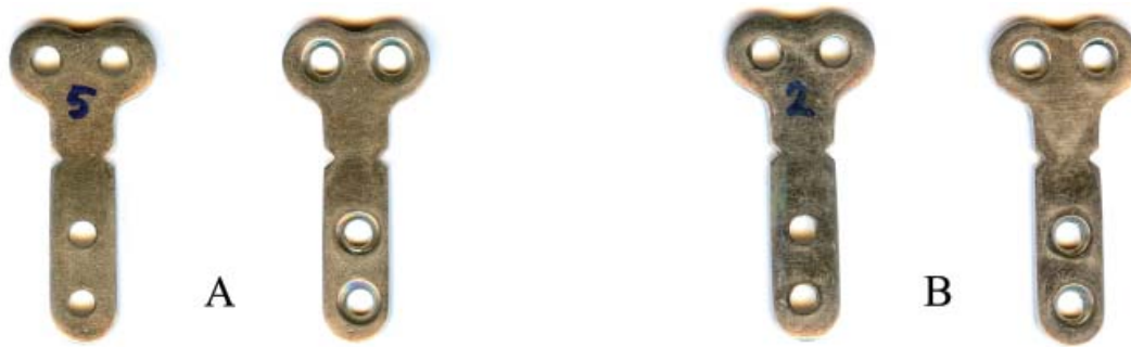
Figure 2 Both surfaces of the 316L stainless T plates fabricated for triple pelvic osteotomy; A: used plates, B: unused plates of the same production batch.
