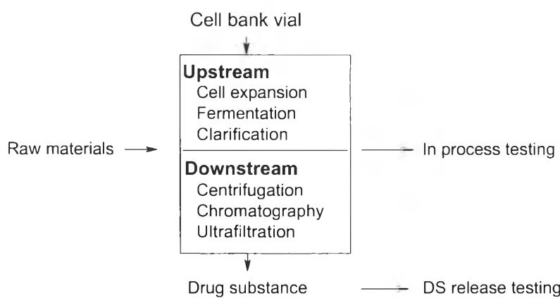
**Figure 2** An outline of biopharmaceutical manufacturing involving upstream and downstream process for drug substance (DS) production
