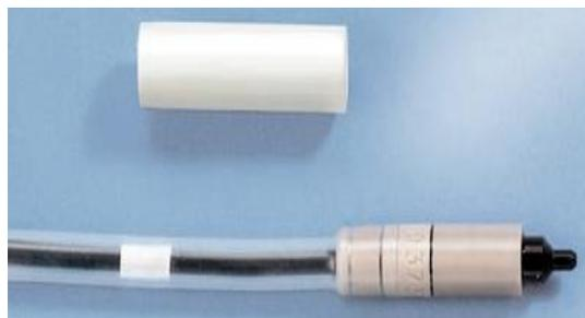
Figure 3.5 IBA CC01 microionization chamber.
