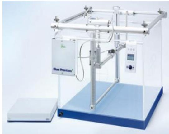
Figure 3.8 IBA blue water phantom.
