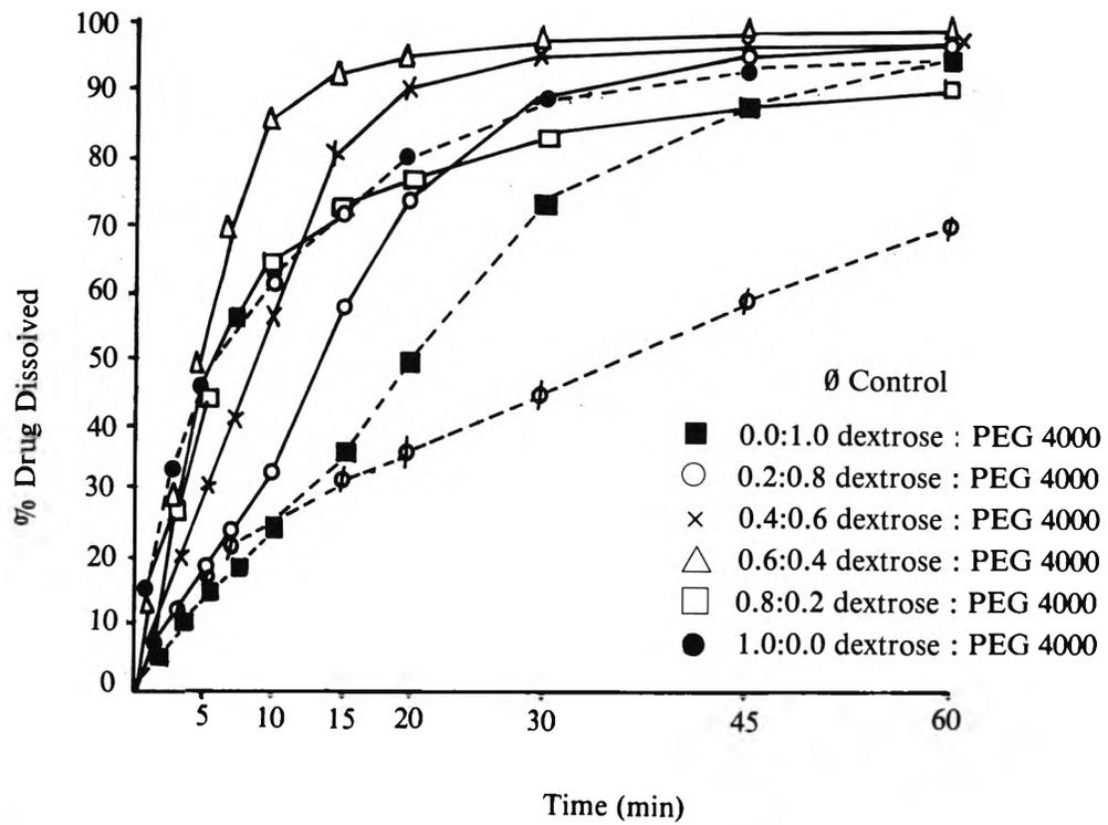
**Figure 1** Dissolution profiles of tablets containing various systems of 1:1 indomethacin : (dextrose + PEG 4000) coprecipitates.
