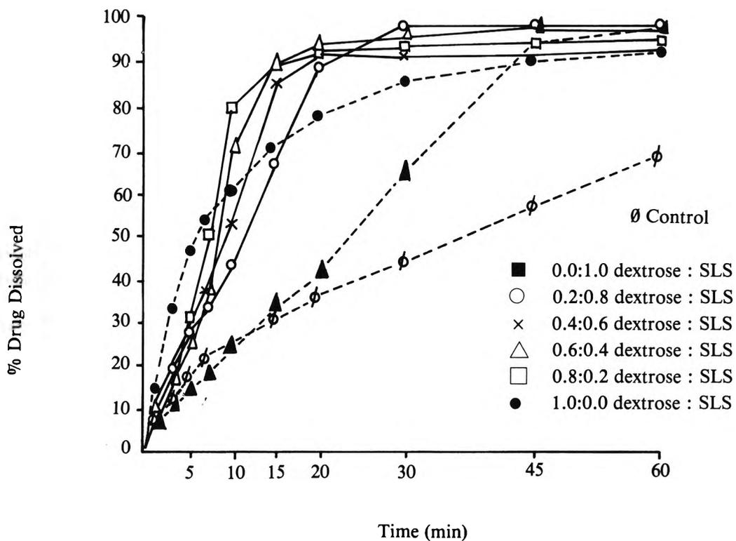
**Figure 3** Dissolution profiles of tablets containing various system of 1:1 indomethacin: (dextrose + SLS) coprecipitates.
