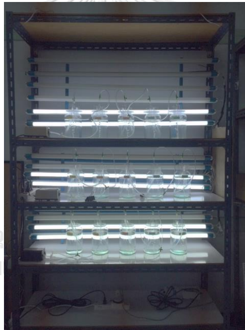
Figure 7 Experimental unit of diatom culture for highest growth, total lipid content and fatty acid composition
