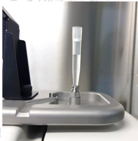
Figure 13 Connection of the pipette tip at the inlet port of MFI™ instrument
