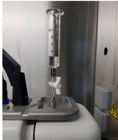
Figure 12 Connection of the syringe at the inlet port of MFI™ instrument
