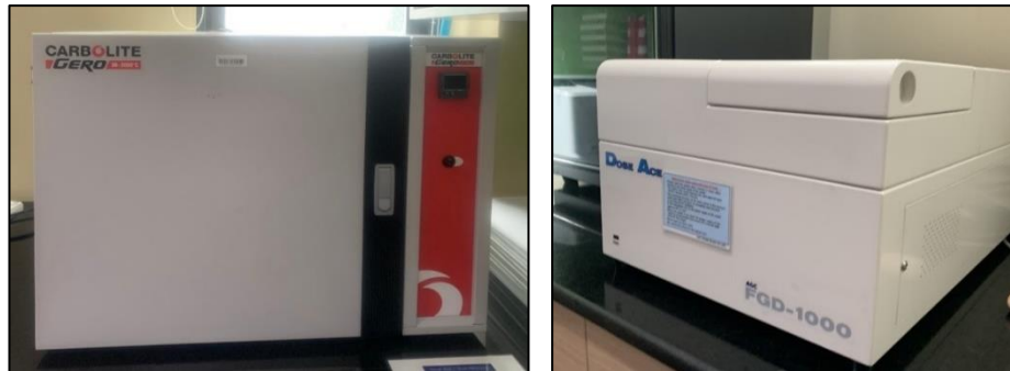
Figure 4.4: Laboratory oven (Carbolite Gero), (Left) and glass dosimeter reader (FGD-1000), (Right)
