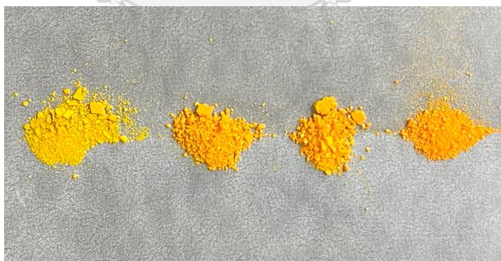
Figure 8 Depicts the color of pure \text{CsPbBr}_3/\text{Cs}_4\text{PbBr}_6 after synthesis, under drying conditions at 80°C for 2 h, at different synthesis temperatures: 95, 110, 125, and 140°C, respectively, from left to right.
